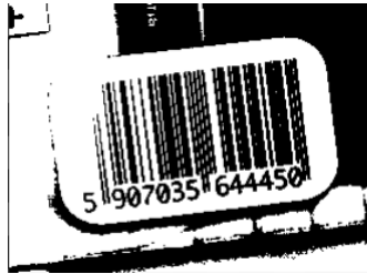
Result of ThresholdImage - the bars can not be recognized.
