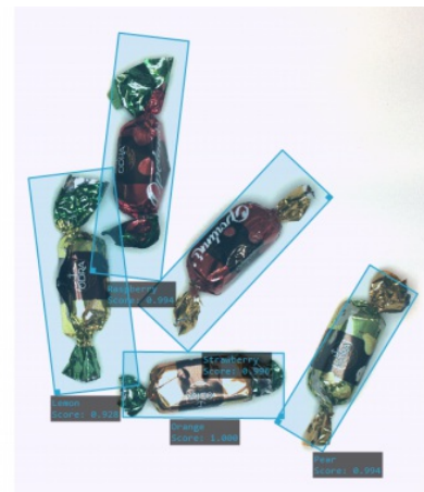
An example of instance segmentation using AvsFilter_DL_LocateObjects tool. Left: The original image. Right: The resulting list of detected objects.
